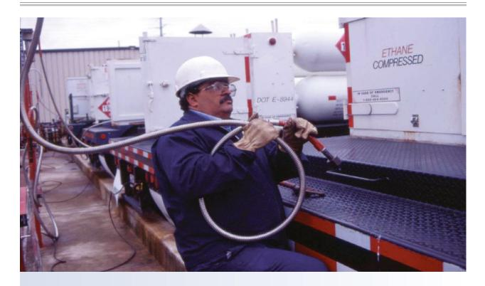
All tube trailer hoses are specifically designed with higher working pressures and smoother inner cores for faster flow. The maximum allowable working pressure and the date of manufacture are permanently marked on each assembly. Armor casing is recommended for all hoses with a wire braided exterior.
